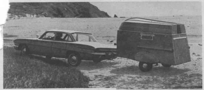
CAMPER-SLEEPER-BOAT is two-wheel fiber-glass trailer with sleeping compartment for two inside and entrance through side door. Tailgate drops down to serve as work table and expose kitchenette containing stove, icebox, and storage for groceries. Nested on top is an eight-foot fiber-glass boat. Cost, \$895. Trailorboat Engineering Co., 923 Francisco Blvd., San Rafael, Calif.
